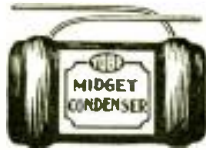
New Tobe midget condenser for all by-pass circuits. Working voltage—600 volts D.C. Test voltage — 3000 volts D.C. Capacities .001 mfd. to .1 mfd.
